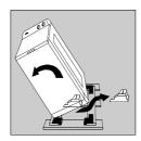
Remove all packing from the washing machine. Tilt the washing machine sideways and then remove the packing under the motor, and straighten the washing machine.
